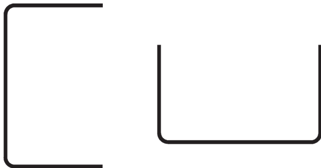
Fig. R2.3b—U-shaped transverse reinforcement.
